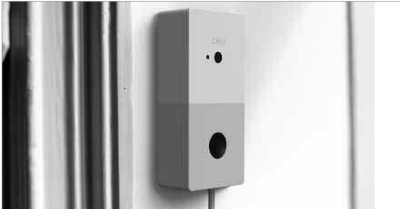
Ring the Chui doorbell activates a camera that takes a picture of visitors and sends it to the homeowner's cellphone.
